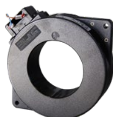
Toroidal transformer. Important: The copper braid of the cable's shield must be insulated and crossed again inside CT's and toroidal transformer's hole
