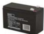
voltage: 12 V = capacity: 7.2 Ah = weight: 2.2 kg = terminal: faston 6.3 mm = optimal lifetime: 5 years = dimensions: 151 × 65 × 94 mm = packaging: 1 pc
