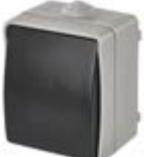
product: cross switch no. 7 = voltage: 250 V~/10 AX = type of mounting: on the wall = version: 1 button = IP rating: IP54 = colour: grey-black = packaging: 1 pc, PE packet
