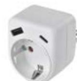
product: adapter plug 1× + 1× USB-A + 1× USB-C = voltage/current: 250 V~/16 A max. = children protection = IP rating: IP20 = material: plastic = packaging: 1 pc, hanging
