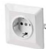
product: single socket with protective side contact = design: SCHUKO = voltage: 250 V~/16 A max. = type of mounting: into a box = version: single = IP rating: IP20 = colour: white (gloss) = packaging: 1 pc, hanging
