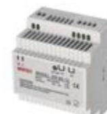
max. output total: 12 V/5 A = input voltage: 100–240 V~, 47–63 Hz = protection against overload, overvoltage and short circuit = designed for: universal = LED indicators = output voltage: 12 V DC = output current: max. 5 000 mA = power supply type: no cable = dimensions: 77 × 55 × 92 mm = packaging: 1 pc, paper box
