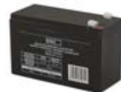
voltage: 12 V = capacity: 7.2 Ah = weight: 2.2 kg = terminal: faston 4.7 mm = optimal lifetime: 5 years = dimensions: 151 × 65 × 94 mm = packaging: 1 pc
