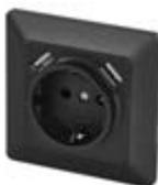
product: single socket with protective side contact and USB output 2.1 A max. = design: SCHUKO = voltage: 250 V~/16 A max. = type of mounting: into a box (recommended depth min. 40 mm) = version: single = IP rating: IP20 = colour: anthracite = packaging: 1 pc, PE packet
