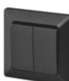
product: double two-way switch 6+6 (5B) = voltage: 250 V~/10 AX = type of mounting: into a box = version: 2 buttons = IP rating: IP20 = colour: anthracite = packaging: 1 pc, hanging
