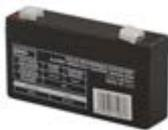
voltage: 6 V = capacity: 1.3 Ah = weight: 0.3 kg = terminal: faston 4.7 mm = optimal lifetime: 5 years = dimensions: 97 × 24 × 51 mm = packaging: 1 pc
