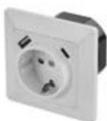
product: single socket with protective contacts and USB output 3 A max. = design: SCHUKO = voltage: 250 V~/16 A max. = type of mounting: into a box (recommended depth min. 60 mm) = version: single = IP rating: IP20 = colour: white (gloss) = packaging: 1 pc, PE packet
