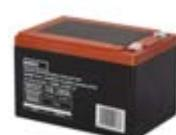
voltage: 12 V = capacity: 15 Ah/20 hrs (14 Ah/10 hrs, 12 Ah/2 hrs) = weight: 4.25 kg = terminal: faston 6.3 mm = optimal lifetime: 4 years for cyclic operation (approx. 1 200 cycles for 30 % D.O.D = discharge depth) = dimensions: 150 × 100 × 102 mm = packaging: 1 pc
