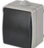
product: switch controller (1/0) = voltage: 250 V~/10 A = type of mounting: on the wall = version: 1 button = IP rating: IP54 = colour: grey-black = packaging: 1 pc, PE packet
