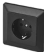
product: single socket with protective pin and child safety cover = design: SCHUKO = voltage: 250 V~/16 A max. = type of mounting: into a box = version: single = IP rating: IP20 = colour: anthracite = packaging: 1 pc, hanging
