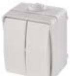
product: serial switch no. 5 (chandelier) = voltage: 250 V~/10 AX = type of mounting: on the wall = version: 2 buttons classic water-resistant = IP rating: IP54 = colour: white = packaging: 1 pc, PE packet
