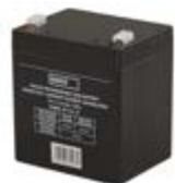
voltage: 12 V = capacity: 4.5 Ah = weight: 1.46 kg = terminal: faston 4.7 mm = optimal lifetime: 5 years = dimensions: 91 × 71 × 105 mm = packaging: 1 pc
