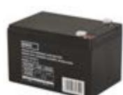
voltage: 12 V = capacity: 12 Ah = weight: 3.3 kg = terminal: faston 6.3 mm = optimal lifetime: 5 years = dimensions: 151 × 98 × 96 mm = packaging: 1 pc
